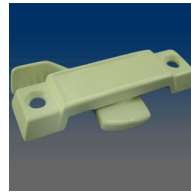
MODEL:3160LH Sweep lock, left, 2.244" C/L, .38" throw, #8 screw, .39" setback.
