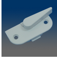
MODEL:9826 Sash lock, flush mount, 1.68" C/L, .575" set back, #8 screw, recessed, with straight handle, others are same as 9821
