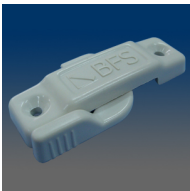
MODEL:31624BF Composite sweep lock, 2.25" C/L, .31" beveled throw, #6 screw, .43" setback, round housing with "BFS" logo, tongue with nibs, with glossy finish
