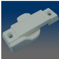
MODEL:31776 Composite sweep lock, 2.25" C/L, .53" throw, #10 screw, .39" setback, squared housing, tongue with ribs, with glossy finish
