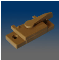
MODEL:3410 Sash lock, surface mount, 2.062" C/L, .438" setback, #6 screw, nesting nib, flat handle design
