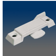
MODEL:3170 Sweep lock, 2.244" C/L, .50" throw, #8 screw, .39" setback
