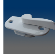
MODEL:9828 Sash lock, flush mount, 1.68" C/L, .575" set back, #8 screw, with beveled cam, others are same as 9820
