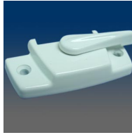
MODEL:9417 Sash lock, surface mount, 2.062" C/L, .438" set back, #6 screw, nesting rib, match with 9317 keeper
