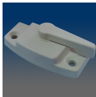
MODEL:32982 Composite sash lock, 2.188" C/L, .73" setback, #12 screw, with powdered coating
