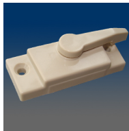
MODEL:32801 Composite sash lock, 2.25" C/L, .39" setback, plastic housing, zinc cam, non-powder coated version
