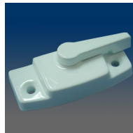
MODEL:32262 Composite sash lock, surface mount, 2.062" C/L, .688" setback, #6 screw, match with 82262 keeper
