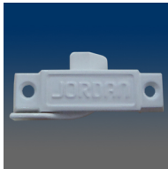
MODEL:3163JD Sweep lock, 2.25" C/L, .38" throw, #10 screw, .38" setback, with molded logo "Jordan"
