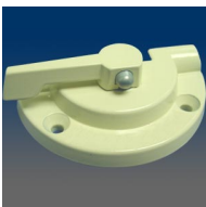
MODEL:9205RB Sash lock, surface mount, 1.88" C/L, .688" set back, #6 screw, half round housing, metal push button handle release
