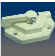
MODEL:9205SB Sash lock, surface mount, 1.88" C/L, .688" set back, #6 screw, square housing, metal push button handle release
