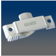
MODEL:3170GK Sweep lock, 2.244" C/L, .50" throw, #8 screw, .39" setback, with pad logo "GALKOS"
