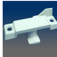
MODEL:3151 Sweep lock, 2.25" C/L, .27" throw, #8 screw, .39" setback
