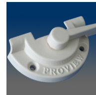
MODEL:9205R-PRO Sash lock, surface mount, 1.88" C/L, .688" set back, #6 screw, half round housing, with logo of "PROVIEW"
