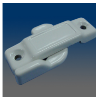
MODEL:31722 Composite sweep lock, 2.25" C/L, .47" beveled throw, #8 screw, .39" setback, round housing, tongue without nibs, with powdered coating
