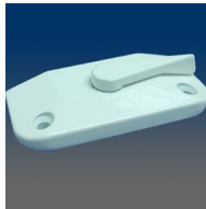
MODEL:9720 Sash lock, surface mount, 2.062" C/L, .688" set back, #6 screw, low profile, hooded
