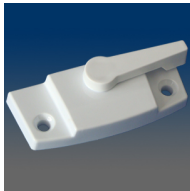
MODEL:32263 Composite Sash Lock, plastic version of 3226SL, 2.062" C/L, .688" setback, housing, handle and cam are made of plastic, match with 8226SL
