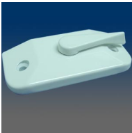
MODEL:9710 Sash lock, surface mount, 2.062" C/L, .438" set back, #6 screw, low profile, hooded
