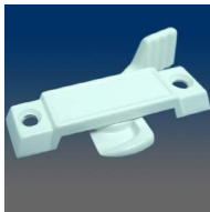
MODEL:3161 Sweep lock, 2.25" C/L, .4" throw, #8 screw, .39" setback
