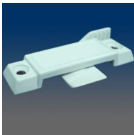
MODEL:3162 Sweep lock, 2.25" C/L, .38" beveled throw, #6 screw, .39" setback
