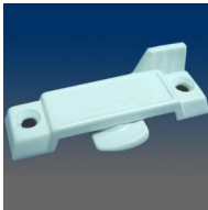
MODEL:3150 Sweep lock, 2.25" C/L, .27" throw, #10 screw, .38" setback
