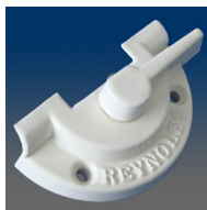
MODEL:9205RB-REY Sash lock, surface mount, 1.88" C/L, .688" set back, #6 screw, half round housing, metal push button handle release, with logo of "REYNOLDS"
