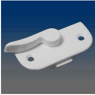
MODEL:9820 Sash lock, flush mount, 1.68" C/L, .575" set back, #8 screw, different lever from 9821
