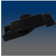
MODEL:3177 Sweep lock, 2.25" C/L, .53" throw, #10 screw, .39" setback, without engraved logo
