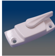
MODEL:9226 Sash lock, surface mount, 2.062" C/L, .688" set back, #8 screw, 9227's housing and 9286's cam
