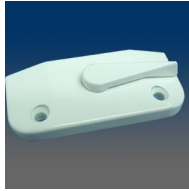
MODEL:9705 Sash lock, surface mount, 1.875" C/L, 1" set back, #6 screw, low profile, hooded
