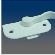
MODEL:9821 Sash lock, flush mount, 1.68" C/L, .575" set back, #8 screw, recessed
