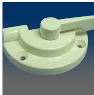
MODEL:9205R Sash lock, surface mount, 1.88" C/L, .688" set back, #6 screw, half round housing
