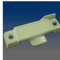
MODEL:3163 Sweep lock, 2.25" C/L, .38" throw, #10 screw, .38" setback
