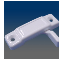
MODEL:31702 Composite sweep lock, 2.25" C/L, .50" throw, .39" setback, #8 screw, round housing, tongue without nibs, with powdered coating
