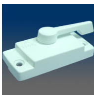
MODEL:3222SK Sash lock, surface mount, 2.062" C/L, .688" setback, #6 screw, flat handle design
