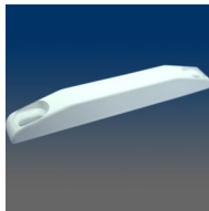
MODEL:9382 Keeper, sash, surface mount, #6 screw, 2.25" C/L, closed back, material: zinc alloy, match with 9280 lock
